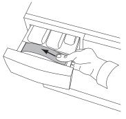
ment, press the card with your thumb and push it sideways (see illustration). The card will then bend slightly and you can easily remove it.
